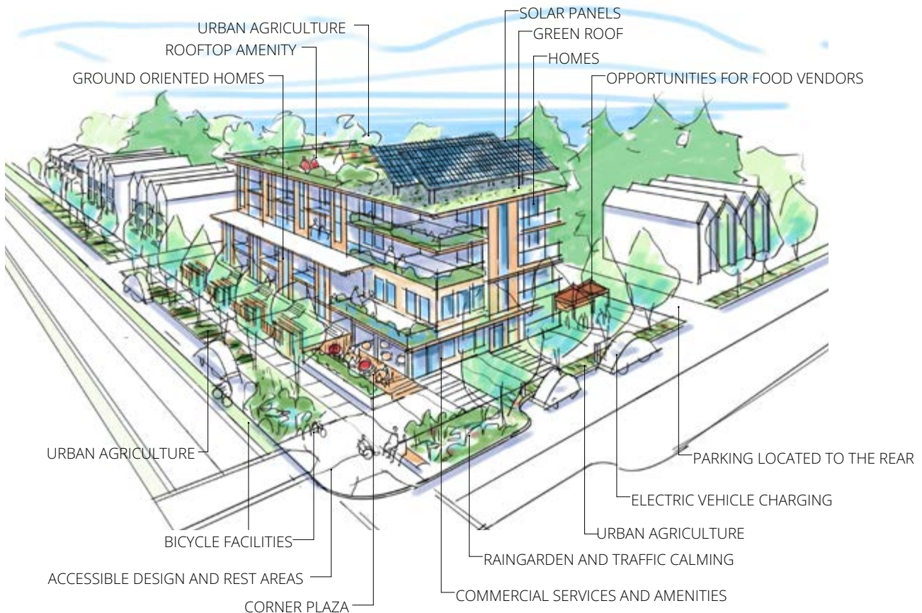
Figure B-4 Artist rendering showing a Neighbourhood Centre. Climate-friendly design opportunities featured.
