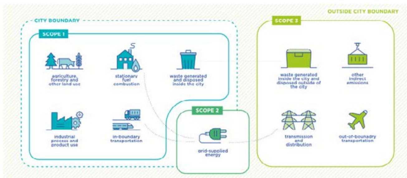
Figure C-2 GPC Emissions Scopes as They Relate to Geographic and Inventory Boundaries. Source: Consumption-based inventories of C40 Cities.
