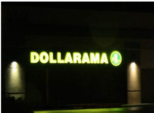
Internally Illuminated Channel Letters
