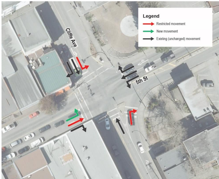
Figure 6-8: 5 th Street and Cliffe Avenue Modifications
